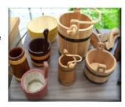
Participants construct a maple sugar keeler using traditional methods and hand tools. Stave construction, head measurement and fitting, metal hoop splaying and riveting will
