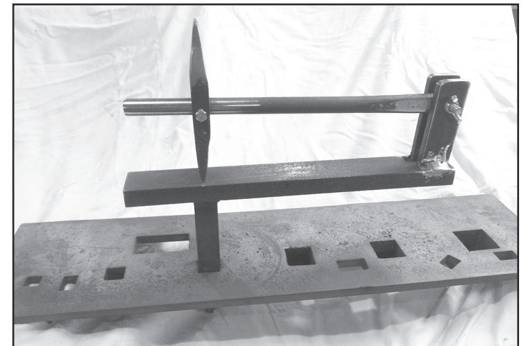
Creasing and forming swage (top) made by Kim Ankeny and Mark Ware for use in a new tinsmithing workshop at the Somerset Historical Center. The bench plate (bottom) was cast from a pattern made by Bill Rearick, a patternmaker by trade but also a talented fiddler and square dance caller for Mountain Craft Days each year.
